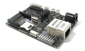
Iboard is a unique Arduino board which features a WIZnet ethernet port, an XBee socket, nRF24L01+ module interface and an ATMega328. This board will add wireless XBee / nRF24L01+ control as well as internet connectivity to your projects. It's great for anything from home automation to robot control. The possibilities are endless!
