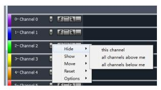
In addition, current channel could be moved up and down through the "Move" menu. "Reset" menu will restore the channels to default settings and labels, and "Options" menu could hide or show the trigger button bar and channel label bar.
