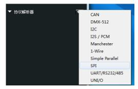
In this dialog, the actual parameter of SPI should be set (Please check section "Standard protocol set" for more details). When this is done, the SPI analyzer would be added. Then the software would analyze the data of channels 0-3 according to standard SPI timing specification, and display the result on channel MOSI and channel MISO.
