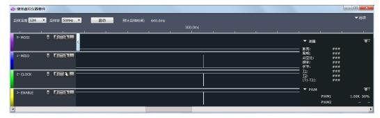
From this figure, we can see the coordinate values of the time axis are too large, and the effective waveform is within a very short period. You can click the left button of the mouse to zoom out the waveform; while the right button would zoom it in. And you can get these done with the mouse wheel too. After the waveform is zoomed up, you could see:
