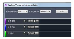
After the trigger is set and the button "start" is pressed again, if the trigger condition (falling edge) we have set have not appeared on channel 0, the logic analyzer would stay in wait state until the falling edge arrives. Then the device will sample and save the data, and upload the data to the computer for displaying and analyzing when the process is complete.
